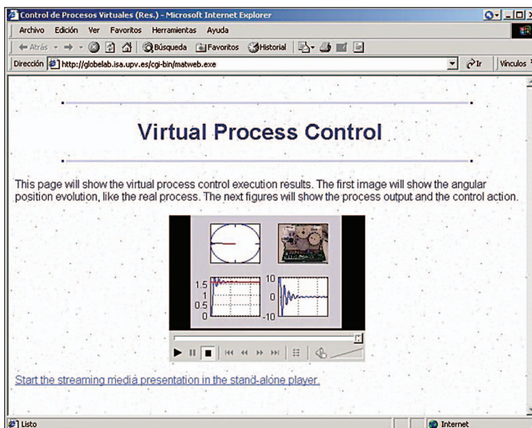
Figure 4. Output page example for a virtual laboratory. The virtual laboratory results processed by the server are sent to an HTML output page. From this output page, learners can either repeatedly execute or download the .avi file, analyzing the system response in a simple, fast, and intuitive manner with a mouse click.
