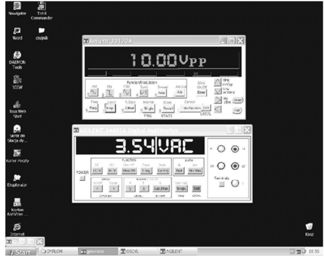
Fig. 7 The front panel of real instrument: function generator Agilent 33120A and digital multimeter Agilent 34401A.
