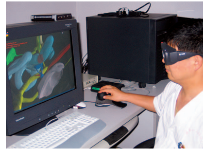
Figure 6. Temporal bone microanatomy virtual laboratory. Using a Spaceball 3D controller, a user manipulates the 3D model in real time.
